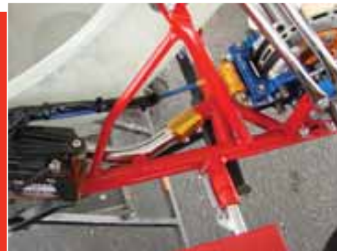
The M32 has a removable 4th sidebar rail, giving you a variety of adjustment options.
