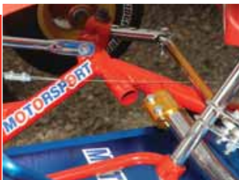
Removable front torsion bar offers two additional connection points on the chassis, providing endless adjustability.
