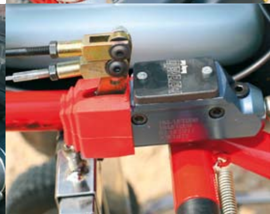
The braking system used in the test is made by K-Kart. It's self-registering, without front discs and with a rear disc in its place almost 2 cm thick.
