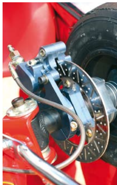
The braking system used in the test is made by K-Kart. It's self-registering, without front discs and with a rear disc in its place almost 2 cm thick.
