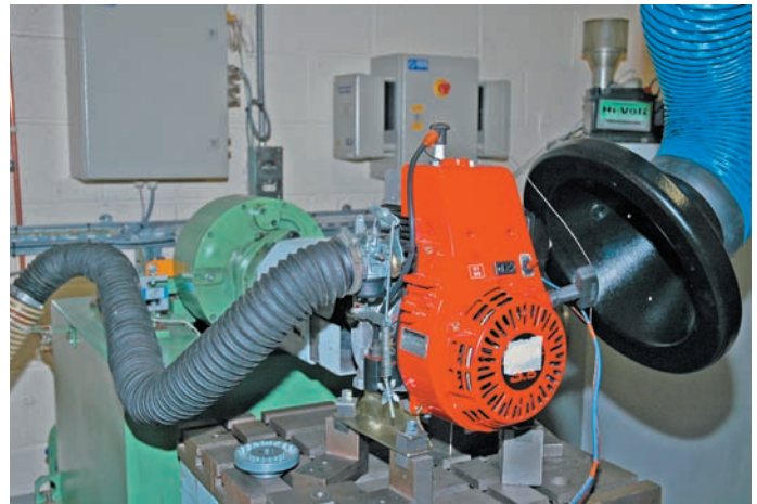
Analysis of engine performance on a dyno
